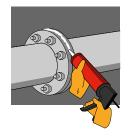
**4.** Extrude the sealant on the seams.
